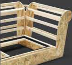
• Frame With Osb - Plywood & Fir
