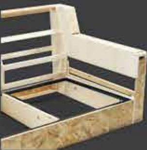
• Frame With Osb - Plywood & Fir
